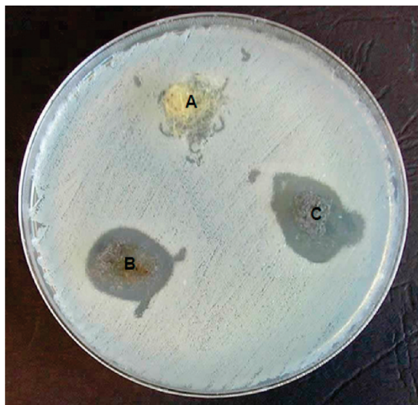
Figure 12. Inhibition zones of S. aureus microbial growth for a silver nanoparticle–merino wool composite: (A) 20 \mu\text{L} of 1% w/w TSC; (B) 10 \mu\text{L} of 10% w/w TSC; (C) 50 \mu\text{L} of 10% w/w TSC.
